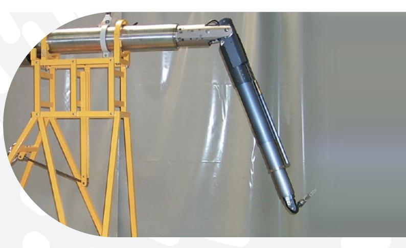
NuPYTHON is a high-radiation resistant, electrically powered and electrically controlled robotic arm capable of performing a variety of tasks in nuclear environments. With 6" and 10" port diameters available, NuPYTHON is capable of being installed
